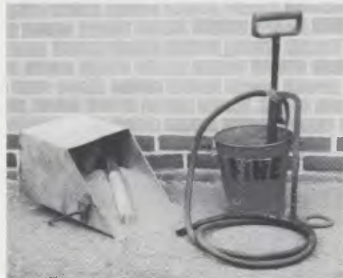
A firewatcher would pick up the burning bomb with a special shovel and place it in a bucket of sand, where it would burn harmlessly. A simple stirrup pump would be used to put out any fire that had been started by the bomb on a wooden roof.
